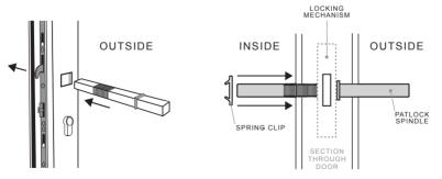
Hold the PATLOCK spindle firmly from the outside and push the spring clip onto the PATLOCK spindle from the inside of the door ensuring that the clip engages with the grooved section to secure in position.
